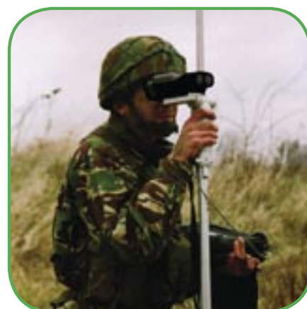
LaserAce® 300 used with Encoder where higher accuracy horizontal angle measurements are required
