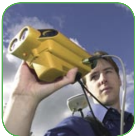
LaserAce® 300 can be integrated with any type of GPS for GPS offsets
