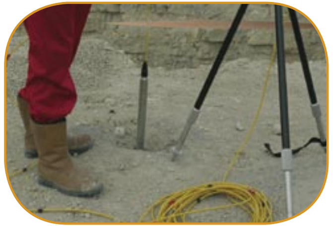
Boretrak® being lowered by hand into borehole
