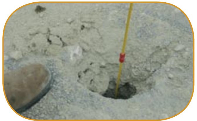
Markers on the cable indicate each metre
