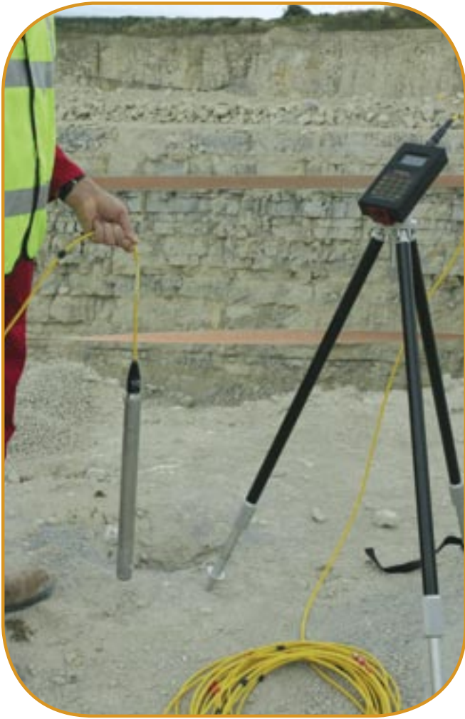
Boretrak® showing complete system including tripod mounted CDU logger'
